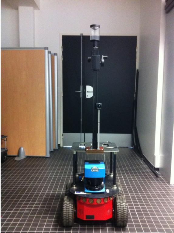
Figure 1: Pioneer 3-AT mobile robot with mounted catadioptric sensor.
