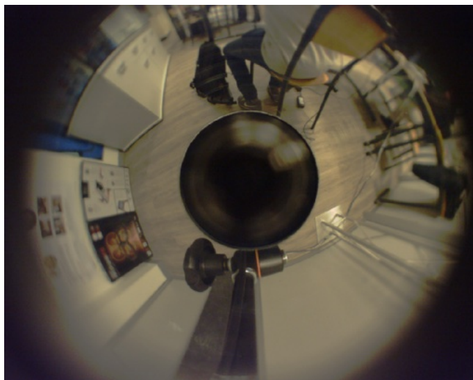
Figure A.1: Image from catadioptric sensor: large unusable area in center.
